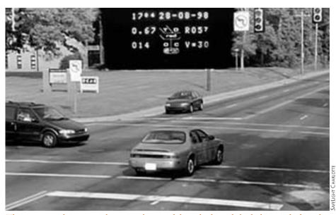
The automated camera takes two photos of the vehicle and the light, one before the vehicle enters the intersection, and one after. Above, the second photo, with relevant data superimposed: "17 04" is the time of the violation; "28-08-98," the date it occurred; "0.67," the elapsed time between the two photos; "R 0 57," the total elapsed time of the red phase at the time of the second photo (here, 5.7 seconds); "014," the violation number on the camera film; and "V = 30," the vehicle speed.
