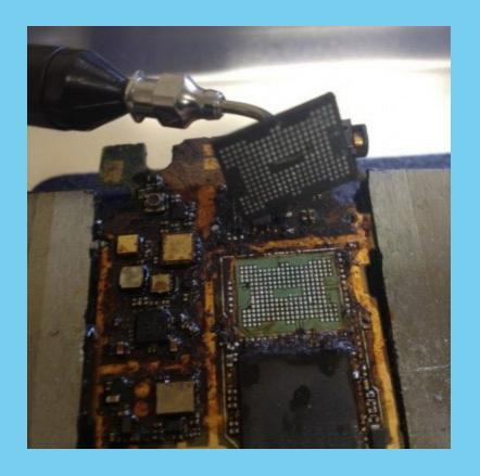
Technique where the flash memory chip is physically removed from the device's circuit board to extract data
